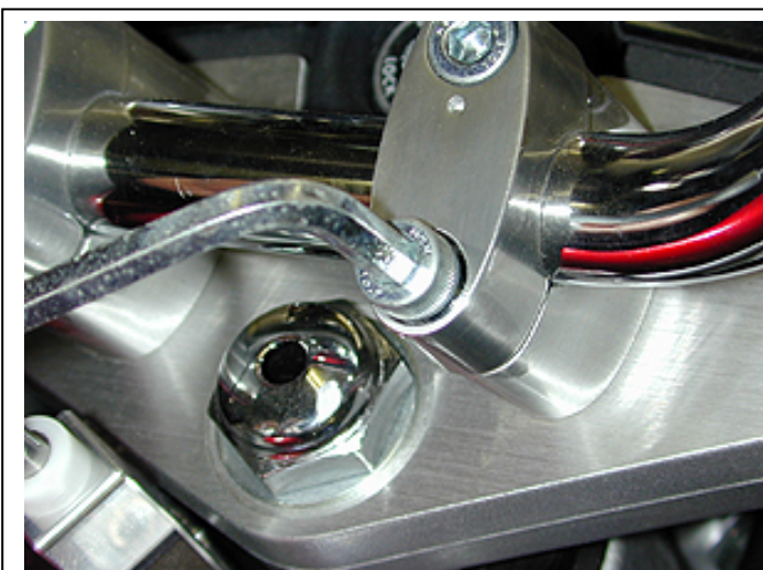
Removing the upper handlebar mount
